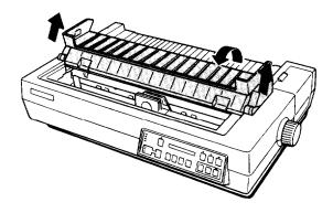
3. Slide the print head to the middle of the printer.
